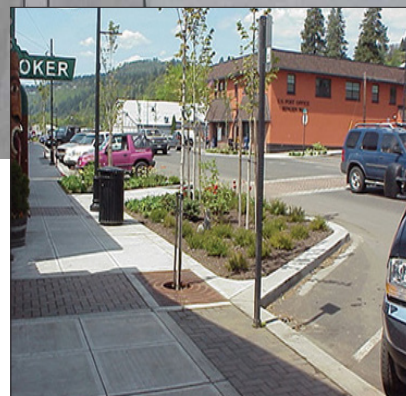
curb extension, Bingen, WA center median refuges, Longmont, CO and Boulder, CO
