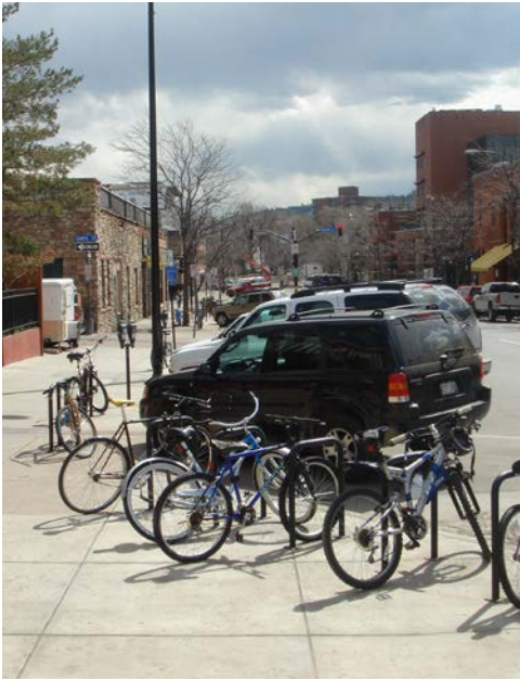
An example of “inverted-U” parking racks located within the sidewalk furnishings zone and on a curb extension, as recommended for installation on side streets within Downtown Sheridan.
