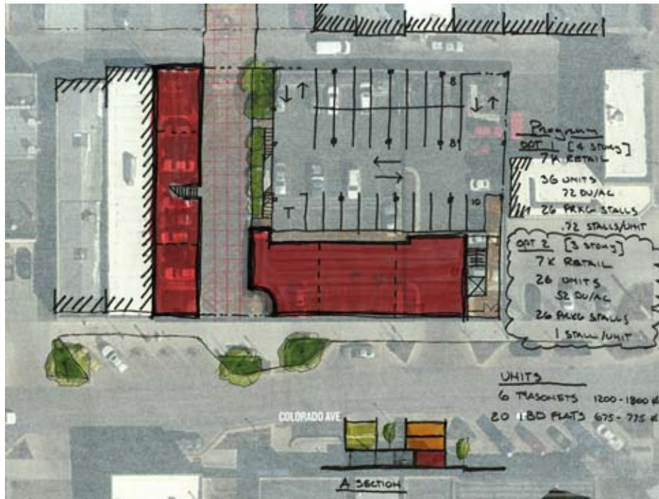
Image 12. Floor plans showing the layout of the potential first level of the Colorado Avenue parking lot development.
