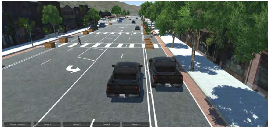
DESIGN #2. Possible LQC intervention to narrow lanes, shorten crossing distances, and stripe unnecessary turn-lane area.
